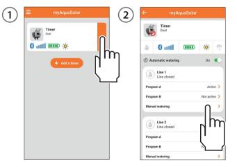
By pressing on the information about the watering run time you can select the run time for manual watering. To start watering, press START.
